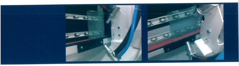
It's possible to work with one or two blast guns mounted on a motorized reciprocator that moves them from bottom to top and vice-versa in the blasting area.
