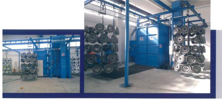
Size of the machine and loading capacity of the hooks depend on the parts to be shot blast. The plant is provided with cartridge or sleeve filter according to the needs.
