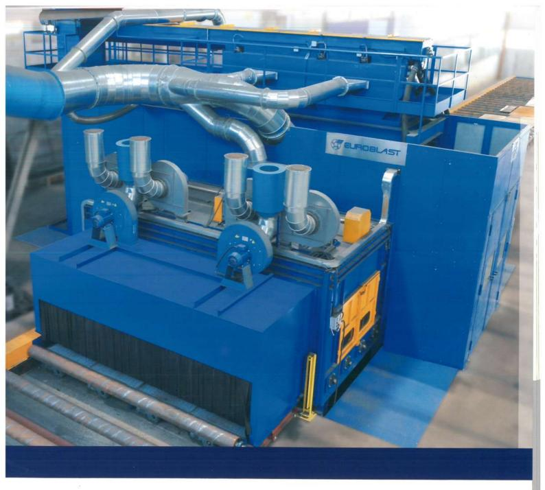
The tunnel blasting machine with roller conveyor is the most suitable plant for the treatment of plates, beams, profiles and structures for components.
